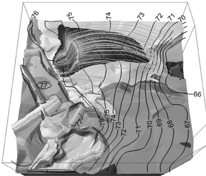
**Fig. 3:** Groundwater flow system in a complex geological structure in the case of the Bitterfeld area. The groundwater contours don not help in construction of the pathways. Only groundwater flow and transport models (based on detailed geological models) yield numerically appropriate results that can be used for the assessment of contaminant spreading.
