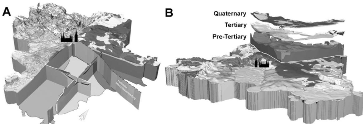
**Fig. 1:** Geological model of Halle / Saale. Fig. 1A shows virtual cross-sections and the main faults striking through the city. In Fig. 1B the distribution of 24 individual layers, e.g. aquifers and aquitards, is visualized to give insight to potential aquifer connections and layers with high adsorption capacities.
